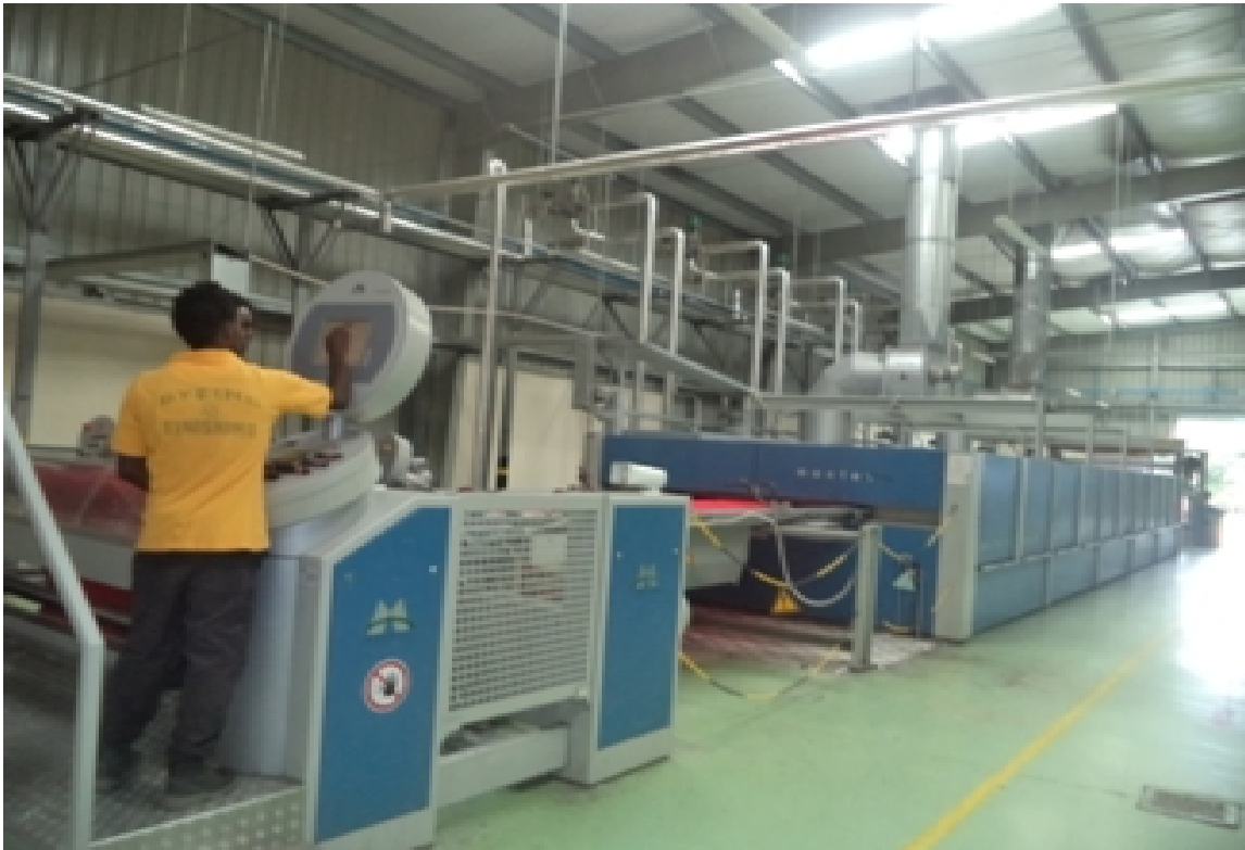
DYEING Section installed in factory owned and managed by the Government as per contract is 100% fully functional. The machine comes from Germany, Tensionless dryer, Steiner & Com
