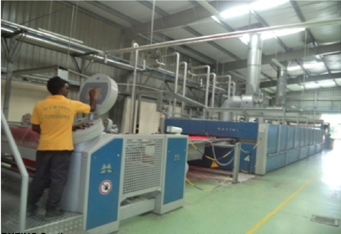
DYEING Section with the different machinery installed with the equipment as per demand. 100% and 100% of the machinery is from Germany, Tensionless dryer, Steiner & Com
