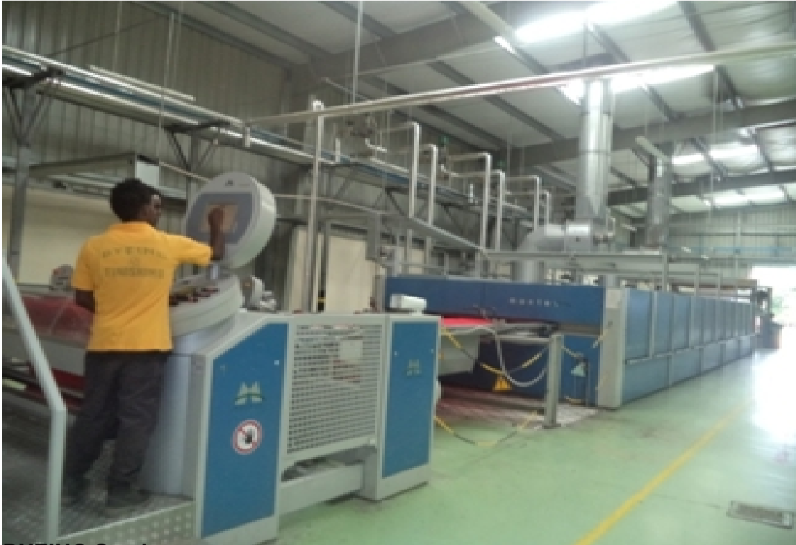
DYEING Section of the dyeing process where the fabric is dyed with the dye. The dye is a chemical which is 100% and the dyeing is done in the dyeing machine. The dyeing machine is a tensionless dryer, Steiner & Com
